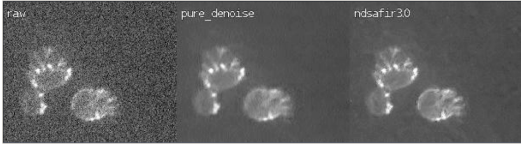
FIGURE 3 – Comparisons of two multiframe denoising methods. Left : original image; middle : wavelet-based method [172]; right : patch-based method [137].
