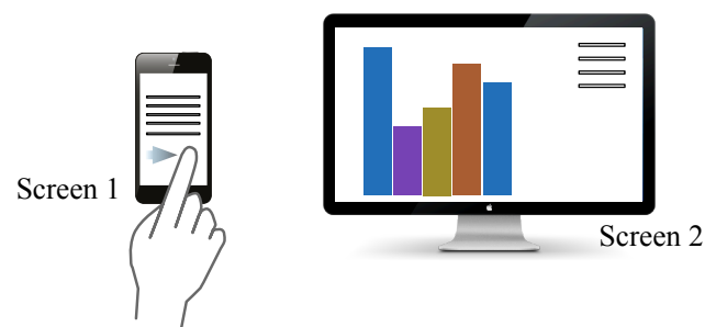
Figure 3. Shows an example for the swipe gesture in combination with the active edges for a ‘Multi Screen’ setting.
