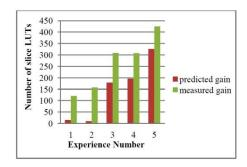
Figure 4: Prediction of the occupancy gain with merging
