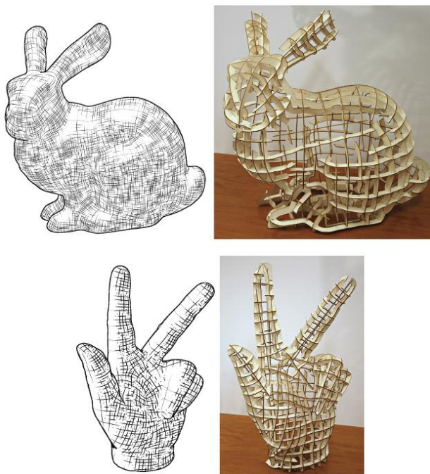
Figure 1: Starting from a 3D model with a cross field the Mesh Joinery approach allows to automatically generate flat cut arrangements that well approximate the original shape.
