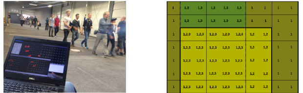
Figure 5: Airport experiment: live snapshot of the central control (left), camera coverage of the area (right). Camera 1 is the infrared camera, cameras 2 and 3 are Kinect cameras. Table 1: Mean relative and absolute errors \delta x/\Delta x for airport experiments with infrared and Kinect cameras.
