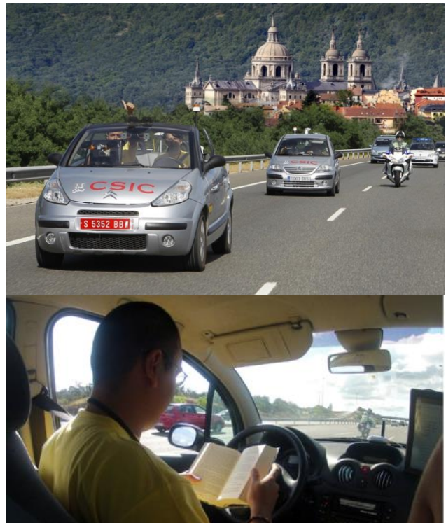
Fig. 9. Demonstration on the motorway. Upper image: Clavileño and Platero during the experiment. Bottom image: Inside the trailing vehicle, showing the "driver" reading a book.
