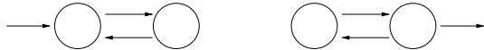
Fig. 2. Examples of non-partially reversible queueing networks: the traffic equations do not have a positive solution.
