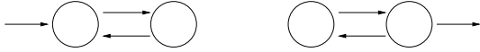
Fig. 2. Examples of non-partially reversible queueing networks: the traffic equations do not have a positive solution.
