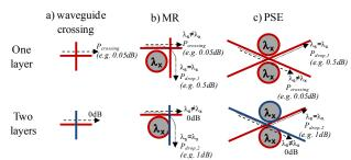
Figure 2: Implementation with one and two layers: a) waveguide crossing, b) MR and c) PSE
