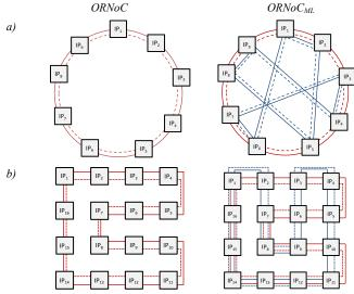
Figure 3: Optical crossbars ORNoC and ORNoC<sub>ML</sub>: a) topology to interconnect 9 IP cores and b) layout for 4x4 IP cores.
