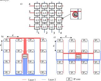
Figure 6: a) Matrix topology, b) layout without waveguide crossings and c) layout with the shortest waveguide length
