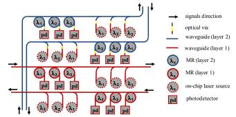
Figure 4: An Optical Network Interface
