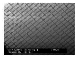
Fig. 9: Real Micro-Mirror Array
