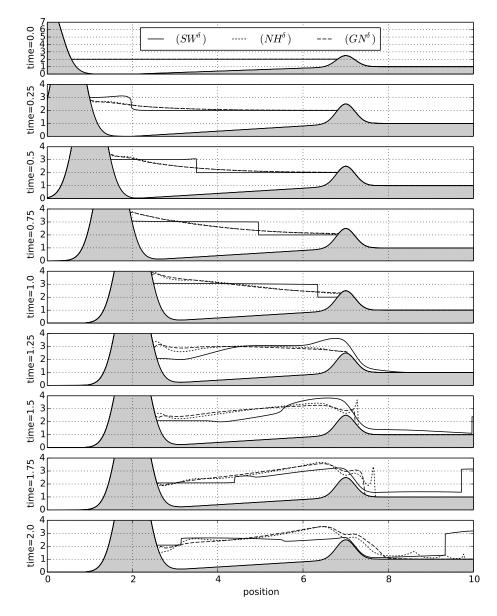
Figure 7: *§*5.4 *Seawall* - Water level approximated by the hierarchy of models at several times.
