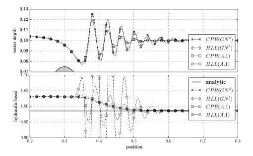
Figure 6: *§***5.3** *Undular jump* - Water level approximated (first line) and hydraulic head (second line) for several schemes.
