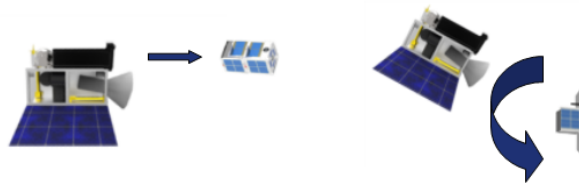
Fig. 3: VBN Experiment. This figure shows the sequence in the VBN experiment: (a) DS-2 CubeSat ejection, (b) VBN manoeuvres.
