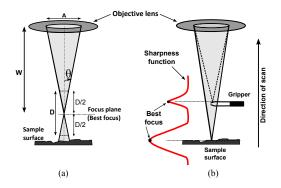
**Figure 1.** (a) SEM focusing geometry (b) sharpness function variation.
