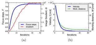
Figure 6. Validation of the method at a magnification of  $\times 300$ : Evolution of (a) focus step and image gradient (b) absolute velocity and working distance during the proposed process.
