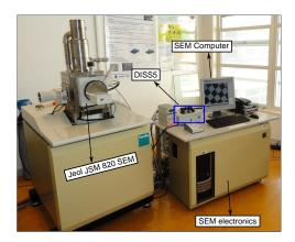
Figure 4. Experimental set-up architecture.
