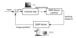
Figure 2. Control framework for SEM autofocus
