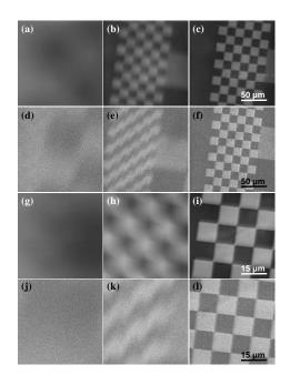
Figure 7. Screenshots obtained during the autofocus process: (a) to (c) with optimal scan speed at  $\times 300$  (d) to (f) with high scan speed at  $\times 300$  (g) to (i) with optimal scan speed at  $\times 900$  (j) to (l) with high scan speed at  $\times 900$ . Last column depict the *in-focus* images.
