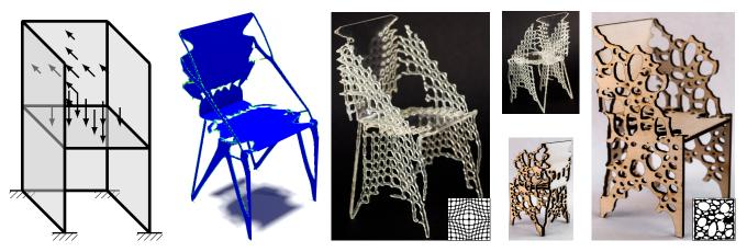
Figure 9: 3D synthesis. From left to right: Boundary conditions, result optimized without appearance, two fabricated chairs from our optimized results using different patterns.
