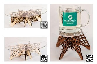
**Figure 13:** Three tables produced with our system, using three planks and structures optimized independently. The two tables on the left use the same external conditions but different patterns. The right table weights 76g and is supporting a filled cup of 762q (10× heavier).
