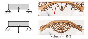
Figure 14: Two structures in MDF wood optimized for different forces but with the same volume constraint. The ratio between the two forces is 10:1. The arrow indicates where the top structure starts to rupture when loaded with the heavier weight intended for the bottom structure (please refer to the accompanying video).
