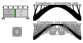
**Figure 8:** Constrained symmetry, with boundary conditions defined on  $\mathbf{x}^*$ . Maximum volume is constrained to 45%.
