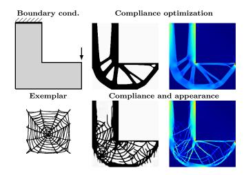
Figure 15: Comparison of Von Mises stresses.  $v_{max} = 40\%$ ,  $\alpha = 1.3$ . We use the classical L-Beam boundary conditions for stress analysis [Duysinx and Bendsøe 1998] (see top left image). Stress colors use the same normalization of both rows. Our structure (bottom row) has a higher compliance ( $\alpha = 1.3$ ), but local stresses are comparable to the ones found in the result without appearance (top row).
