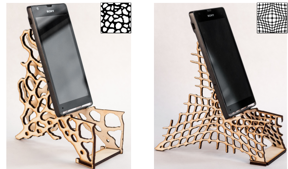
Figure 12: Phone stands fabricated from optimized structures using two different exemplar patterns.
