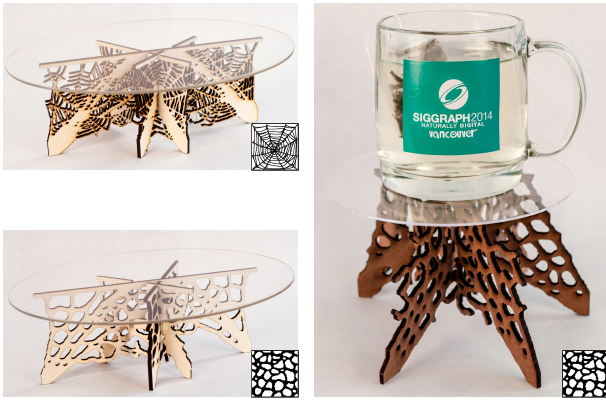
Figure 13: Three tables produced with our system, using three planks and structures optimized independently. The two tables on the left use the same external conditions but different patterns. The right table weights 76g and is supporting a filled cup of 762g (10× heavier).
