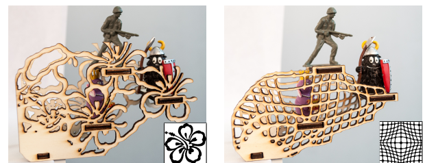
Figure 11: A set of shelves, meant to be fixed on the ground. Two exemplars are used on the same problem, producing results of very different styles but the same purpose.
