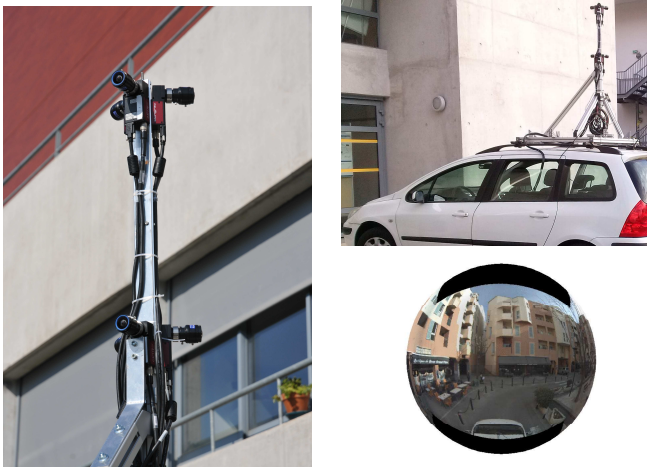
Fig. 4. Globeye stereo sensor and acquisition system.
