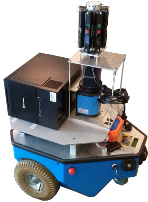
Figure 11: Robot with the omnidirectional RGB-D sensor.
