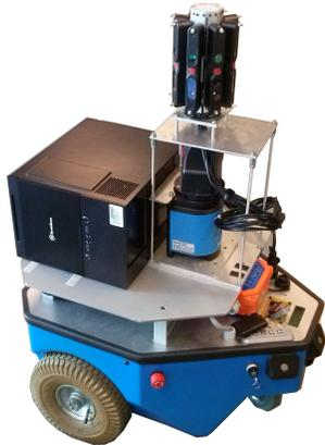
Figure 11: Robot with the omnidirectional RGB-D sensor.
