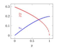
Figure 7: Comparison between our numerical solution (marks) and the analytic one (lines), for the velocity and shear-rate profiles of a Bagnold avalanche flow with  $\mu = 0.5$  and  $\alpha = \tan^{-1}(1.1\mu)$ .
