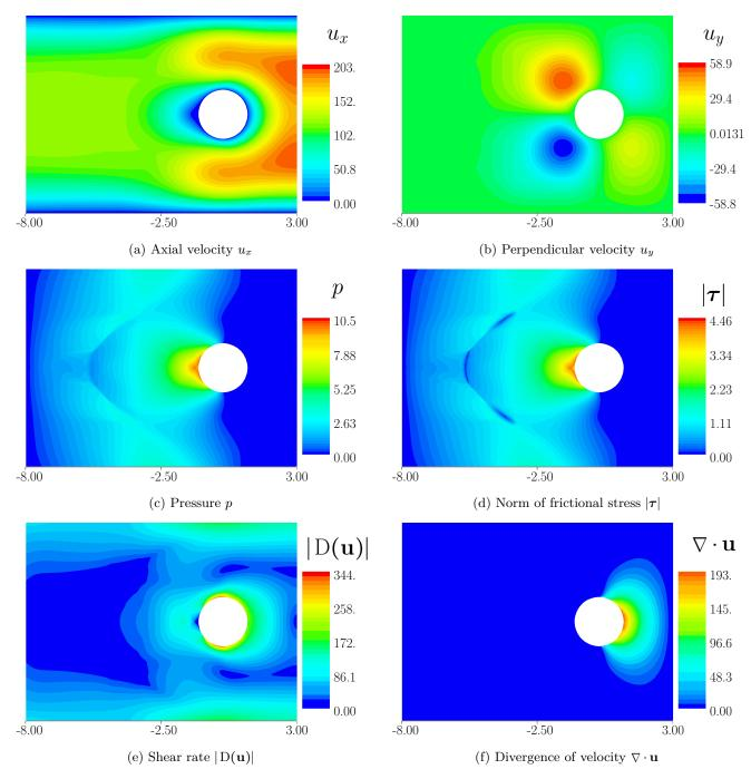
Figure 14: Velocity and stress fields for the flow around a cylinder in a narrow channel, with  $\mu = 0.3$ , Re = 100, Bi = 0 and  $\tilde{D} = \frac{1}{4}$
