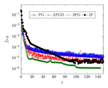
Figure 15: Infinity-norm of the Fischer-Burmeister function as a function of the wall time for the Projected-Gradient, Accelerated Projected Gradient Descent, Spectral Projected Gradient and Interior Points algorithm
