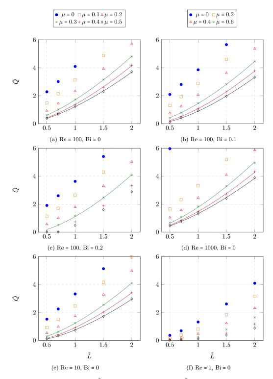
Figure 9: Dimensionless discharge rate  $\tilde{Q}$  versus silo outlet diameter  $\tilde{L}$  for and different rheologies. When  $\mu$  is small, we cannot get a reasonable fit; in the case of the Newtonian flow, the discharge rate is closer to a linear law. Bi mainly influences the k parameter of the law but does suffices to obtain a fit. Large values of Re tend to linearize the discharge rate for small  $\mu$ , smaller values make it quadratic.
