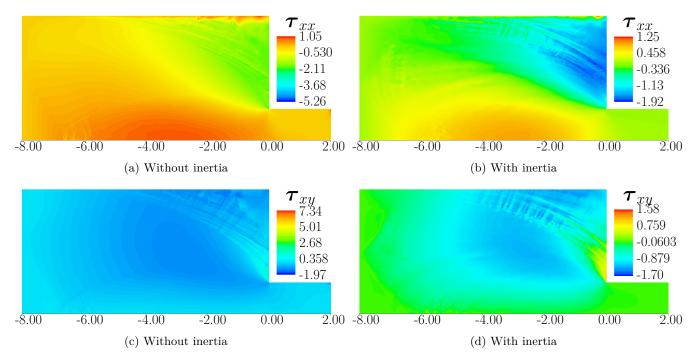
Figure 18: Normal (top) and tangential (bottom) components of the deviatoric stress tensor  $\tau$  for simulations with and without inertia for Re = 100,  $\mu$  = 0.3 and Bi = 0.
