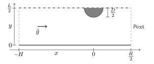
Figure 12: Flow around a cylinder of diameter D in 2D channel of width L. The speed of the flow can be adjusted by varying the external pressure at the downstream boundary  $p_{\text{ext}}$ .
