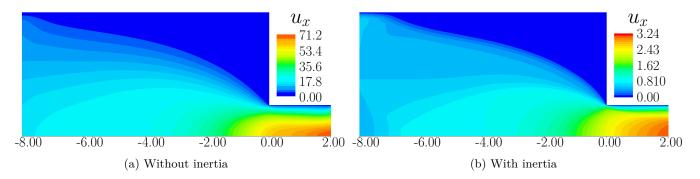
Figure 16: Axial velocity  $u_x$  for simulations with and without inertia for Re = 100,  $\mu$  = 0.3 and Bi = 0.
