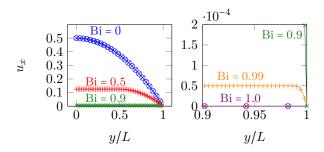
Figure 4: Comparison of the steady velocity profiles  $u_x(-H/2, y)$  between our numerical model using a  $\mathbb{P}_2 - \mathbb{P}_{1d}$  approximation (marks), and the analytic Bingham Poiseuille flow (lines). Plots for high values of Bi (right) are zoomed in compared to plots for lower Bi values (left).
