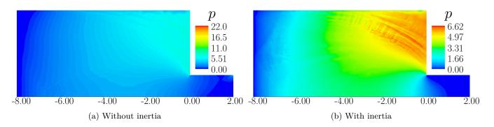
Figure 17: Pressure fields for simulations with and without inertia for Re = 100,  $\mu$  = 0.3 and Bi = 0. In the creeping flow case, there exist a very high pressure point on the boundary of the outlet. In the inertial case, the high-pressure zone on the bottom of the silo starts at some distance from the outlet and is much more widely spread.
