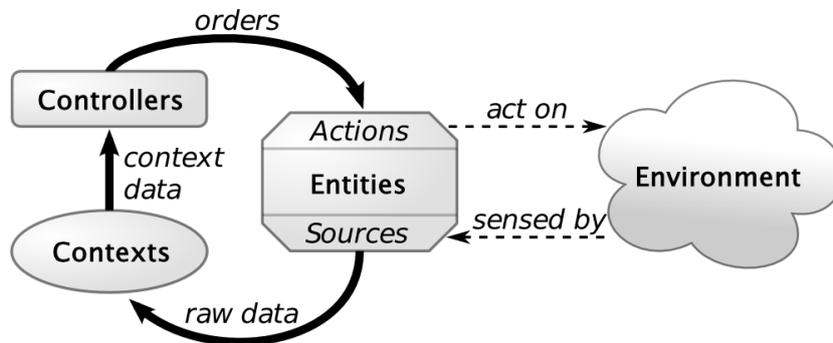
Figure 1: The *Sense/Compute/Control* paradigm, adapted from [6].
