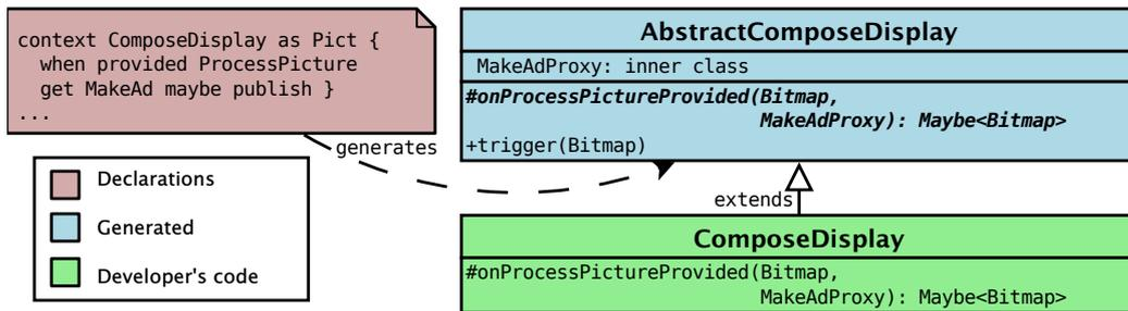
Figure 4: Schematic design of the Java prototype.
