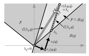
Fig. 7 Geometric interpretation of (114) of the case of  $G_{\mathcal{A}}(q,\dot{q}) < 0$  and  $G_{\mathcal{B}}(q) < 0$ , where (114) has three solutions:  $\lambda_1$ ,  $\lambda_2$  and  $\lambda_3$ .
