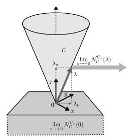
Fig. 2 The friction cone C and its singular-metric normal cones with  $U_{\varepsilon}$  defined by (55). Note that the normal cone at  $\lambda = 0$  is the half-space  $z \leq 0$ .
