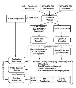
Fig. 1. The ANTAREX Tool Flow
