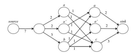
**Figure 4** Example of max-flow graph.
