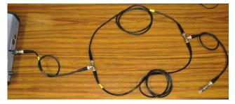
Fig. 1. Composite line including two RG-58 50  $\Omega$  coaxial cables in parallel.
