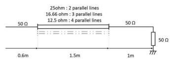
Fig. 2. Topology of the composite lines used. Equivalent cables of characteristic impedance smaller than 50  $\Omega$  are realized by putting multiple 50 $\Omega$  coaxial cables in parallel.
