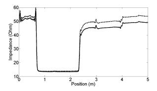
Fig. 4 Comparison of two  $Z_0(z)$  profiles obtained by inverse scattering on the same line including an (equivalent) segment of 25  $\Omega$  with zero padding up to 15 GHz (-) and 30 GHz (--). These results show that a higher zero padding leads to a more accurate result
