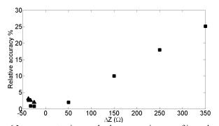
Fig. 6 Inverse scattering method accuracy in case of impedance discontinuities. ( $\blacktriangle$ )Accuracy obtained from the inversion of experimentally measured reflection coefficient. ( $\blacksquare$ ) Accuracy obtained from the inversion of simulated reflection coefficient.
