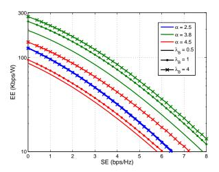
Fig. 9. Multi-cell SE-EE trade-off from  $(P_4)$  as a function of the path loss exponent and the BS density  $(\lambda_B \text{ in points/km}^2)$ .
