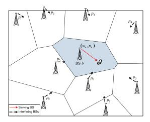
Fig. 2. Example of multi-cell topology with a PPP  $\Phi_{\rm B}$  of 10 cells. The shaded polygon shows the serving area of BS b.
