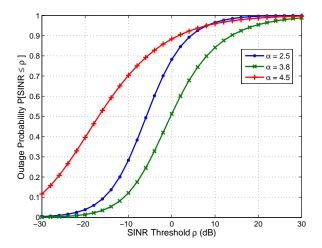
Fig. 7. SINR cdf as a function of the path loss exponent for a user u with  $p_u/w_u=2\mathrm{W/MHz}$ .
