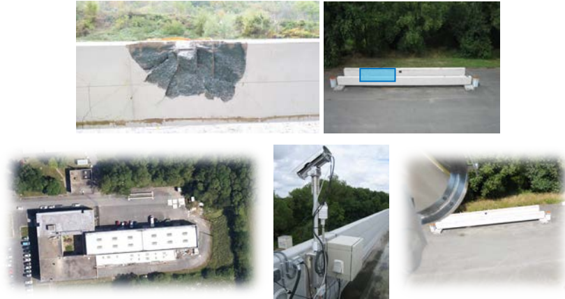
Fig. 6 Long term experiment set-up to monitor 2 reinforced concrete beams in Nantes.
