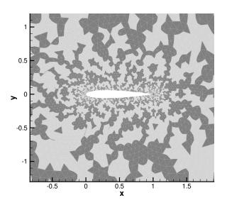
Figure 2: Mesh of Naca0012 for Problem 5.1 with elements randomly subdivided: elements in dark zones are sudivided, the others are not subdivided.
