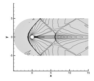
Figure 11: Mach number isolines for test case 5.3.
