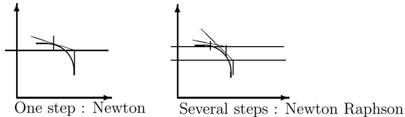
Figure 5: Graphical description of Newton-Raphson iterative method
