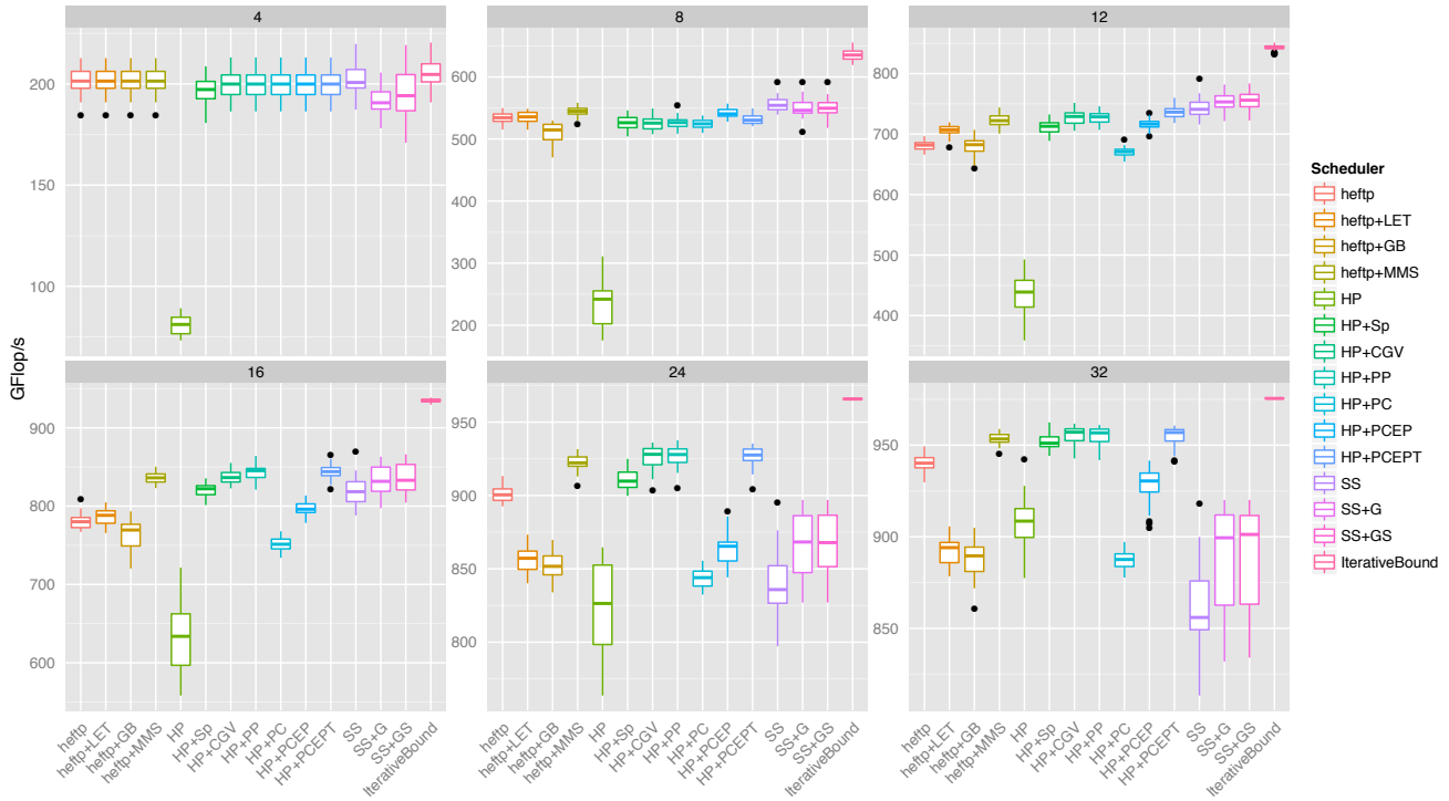
Figure 12. Comparison of different schedulers with perturbed execution timings.
