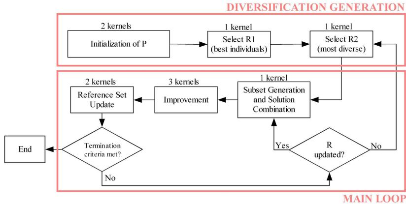
Fig. 1: Block diagram of the Scatter Search Algorithm.
