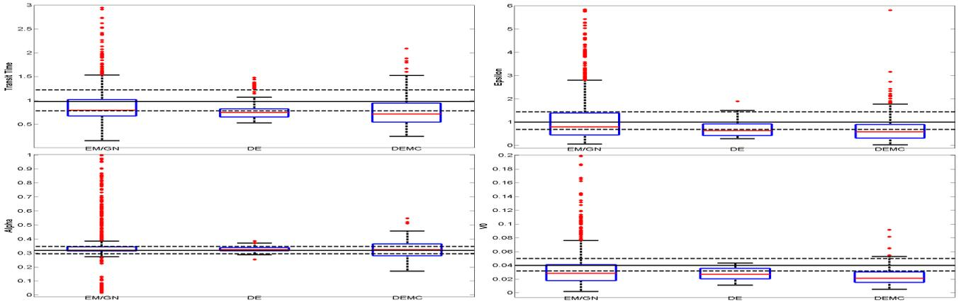
Fig. 2. Boxplots of the EM/GN, DE and DEMC results for  $\varepsilon$ ,  $\alpha$ , transit time ( $tt$ ), and  $V_0$  using globally all real datasets. The parameters prior mean and standard deviation are indicated by the horizontal black lines (solid and dashed, respectively). Since the EM/GN variability is much larger in all cases, we have zoomed-in on a sub-interval for a better visualization.
