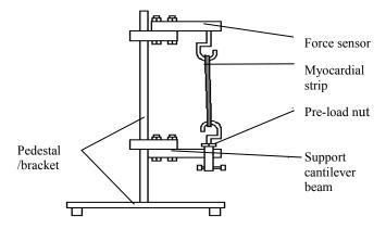
Fig. 1. Schematic of contractile force detecting device
