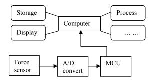
Fig. 2. Frame diagram of data acquisition and processing
