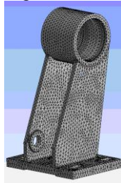
Fig.4. Mesh generation model
