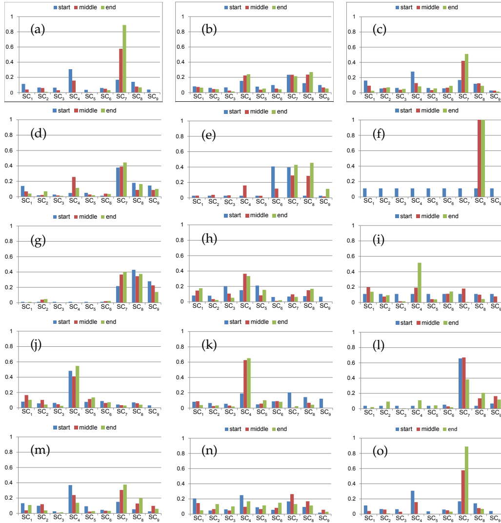
Figure 4: Scagnostics weights over time, where time is split into three generation bins for the start, middle and end of the session; scagnostics types on the x-axes: SC_1 :monotonic, SC_2 : stringy, SC_3 :skinny, SC_4 :convex, SC_5 :striated, SC_6 :sparse, SC_7 :clumpy, SC_8 :skewed and SC_9 :outlying. The plots are for (a) overall, (b) overall success, (c) overall failure, (d–m) successful sessions per participant and (n–o) unsuccessful sessions per participant, all for level-0 of the game.
