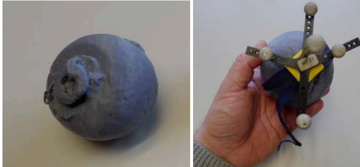
Figure 18. 3D printed weight as tangible interface, with tracking target.
