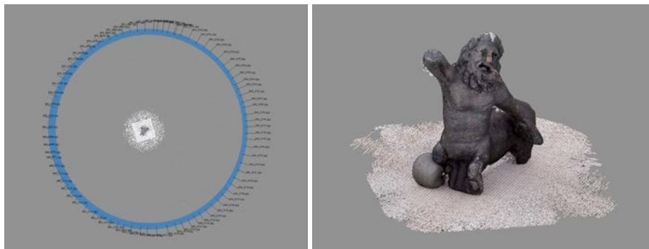
Figure 11. Left: alignment of the photos. Right: dense point cloud.
