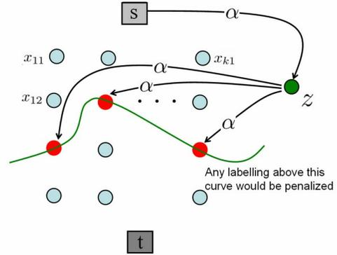
Figure 3. The graph construction for characterizing a general  $k^{\text{th}}$  order multi-label energy function. The variable  $z$  is an auxiliary node that is connected to  $k$  boolean nodes and the source with the same edge cost  $\alpha$ . As a result if all the  $k$  boolean nodes take the label 0 then the cost of the cut is 0. In all other cases there is a uniform cost of  $\alpha$ . This can be seen as a generalization of the graph construction given in [13].
