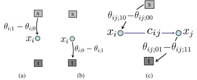
Figure 1. *Converting an energy minimization problem to an st-mincut problem [13]. (a) and (b) show unary potentials are represented using edges in the graph, while (c) shows the same for submodular pairwise potentials.*
