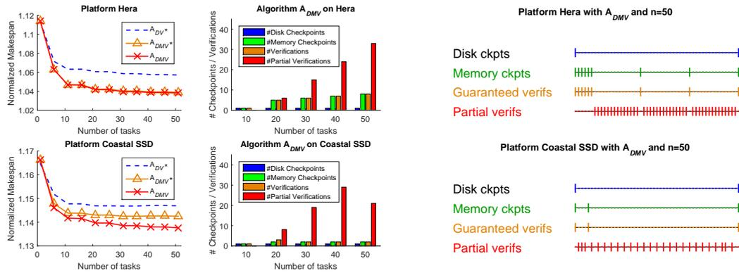
Figure 8: Performance of the three algorithms, and distribution of disk checkpoints, memory checkpoints and verifications (for the  $A_{DMV}$  algorithm) on platforms Hera and Coastal SSD with the *HighLow* pattern.
