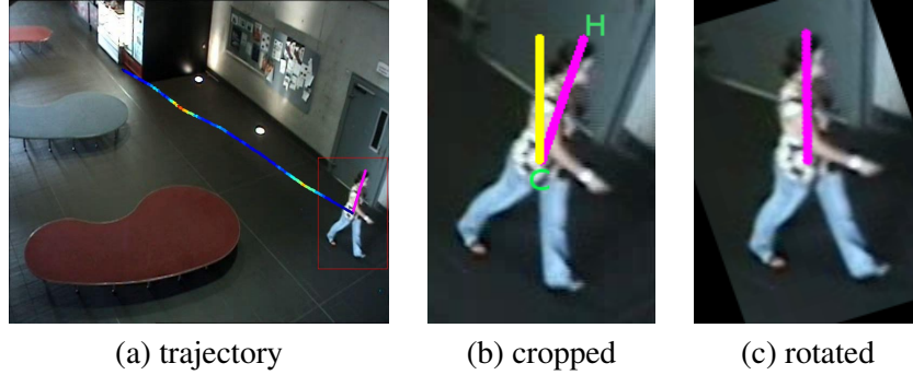
Fig 2: Affine transformation of the target image: (a) trajectory of the target (color of the trajectory illustrates the reliability of the detected pose; see section 4.2 for details); (b) the cropped image obtained by the detection algorithm; (c) the rotated image.
