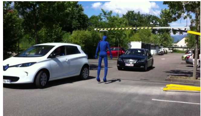
Fig. 15: Real test example of collision detection. The white car blocks the view of a pedestrian (blue) until the last instant when it swerves to the right. The collision detection algorithm installed in the Lexus platform generated alerts about an imminent collision for the driver.
