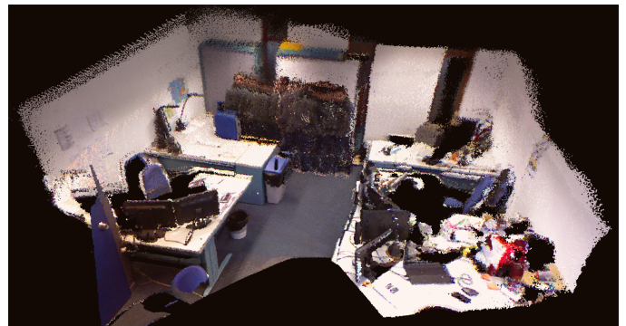
Fig. 2. 3D coloured map produced by our method from a hand-held camera in a dynamic scene. The map displays the static (inliers) and mobile (outliers) vertices. In this image, we aim to show that our method is able to accurately localize the camera when there are moving objects. The accuracy of our method can be inferred from the good quality of the reconstruction of the background (inliers) compared to figure 1.
