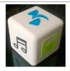
The DomiCube. The DomiCube is a home-made device designed by 5 retired seniors as the result of a 3 hour focus group. It contains an accelerometer and a gyroscope, and is Bluetooth enabled. It sends events when its state changes (e.g., new orientation, top face, and battery level). The DomiCube was built in the Creativity Lab of the EquipEx AmiQual4Home, ANR-11-EQPX-00.
