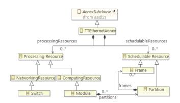
Fig. 2. Overview of AADL-TTEthernet metamodel
