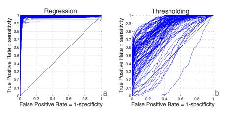
**Fig. 6.** ROC analysis of the tested cases comparing our method (a) to the thresholding of the deformation patterns (b).
