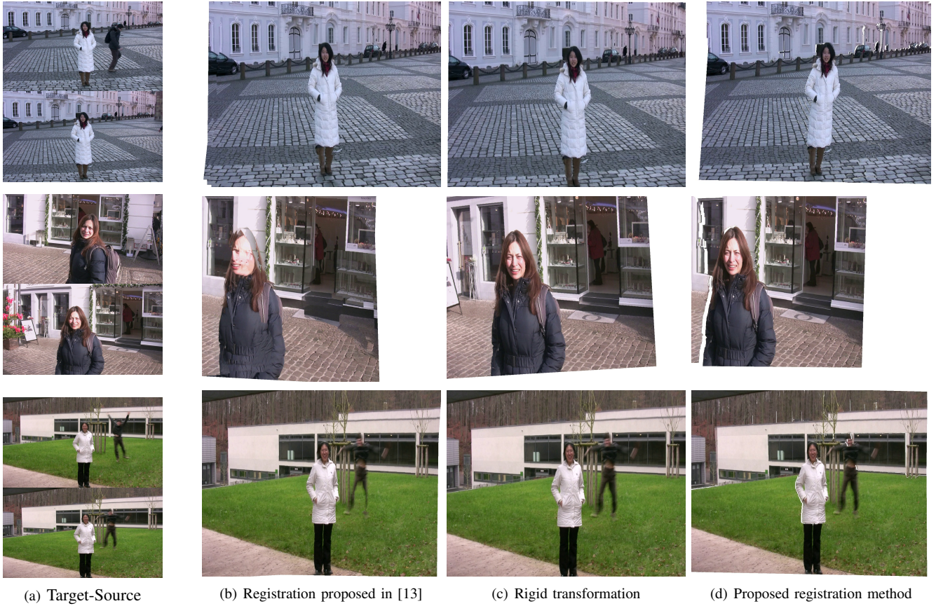
Fig. 6: Comparison of registration quality with scenes having different types of camera motion. First row: slow rotation; Second row: fast view changes; Third row: small view change and zooming. The columns represent: (a) Target and source images are illustrated on top and bottom, respectively; (b) MRF-based registration with epipolar constraints as in [13]; (c) registration using a rigid transform and (d) the proposed method.
