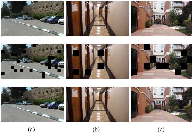
Fig. 16: Sample frames from videos considered for error concealment. (a) Scene11 ; (b) Scene12 ; (c) Scene13 . From top to bottom: Original frames; Frames with the missing blocks; Inpainting results using the proposed approach.
