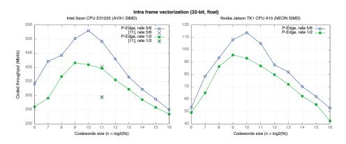
**Fig. 6.** Performance comparison between several code rates of 32-bit floating point decoding stages (running on the Intel<sup>®</sup>Xeon<sup>®</sup>CPU E31225 and, respectively, on the Nvidia<sup>®</sup>Jetson TK1<sup>®</sup>CPU A15).
