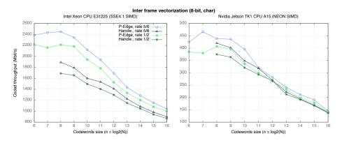
Fig. 7. Performance comparison between several code rates of 8-bit fixed point decoding stages (running on the Intel<sup>®</sup>Xeon<sup>®</sup>CPU E31225 and, respectively, on the Nvidia<sup>®</sup>Jetson TK1<sup>®</sup>CPU A15). Circles show P-EDGE results. Triangles show our former "handwritten" implementation results [8].
