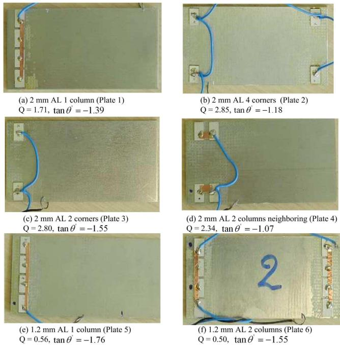
**Fig. 5.** Aluminum resonators with different piezoceramics layouts. The dynamic amplification factor ( $Q$ ) and the piezoelectric loss tangent ( $\tan \theta'$ ) are labeled in each condition.
