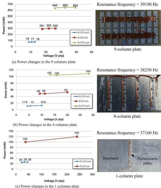
**Fig. 2.** Power changes in the three tactile plates. Piezoceramics were glued on the resonator to excite the resonance vibration. The dimensions for the aluminum resonator were  $76mm \times 41mm \times 1mm$ .
