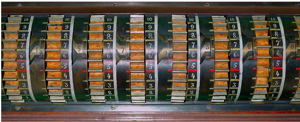
Figure 11: Detail of Chebyshev's first calculating machine. This machine is not correctly mounted. When a figure is 0, the next one should be between two digits, and this isn't the case for the units and tens. Moreover, because the mounting is incorrect, it is difficult to follow the white strips. The first 0 points downwards, but there is no figure downwards in the tens. The third figure is 3, and the next one should then be almost centered, which isn't the case. (picture from http://tcheb.ru )
