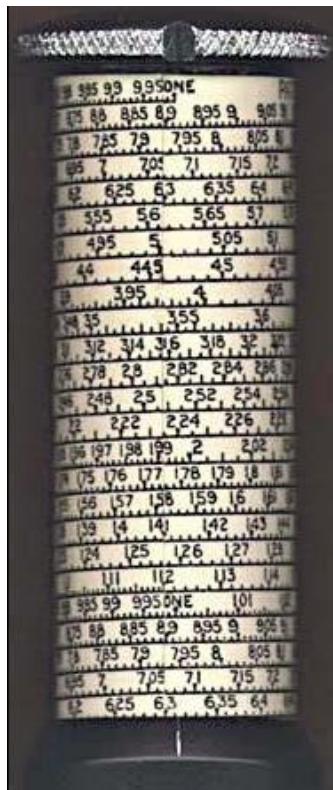
Figure 5: An excerpt of an Otis King slide rule. (Wikipedia, photo by Richard Lyon)
