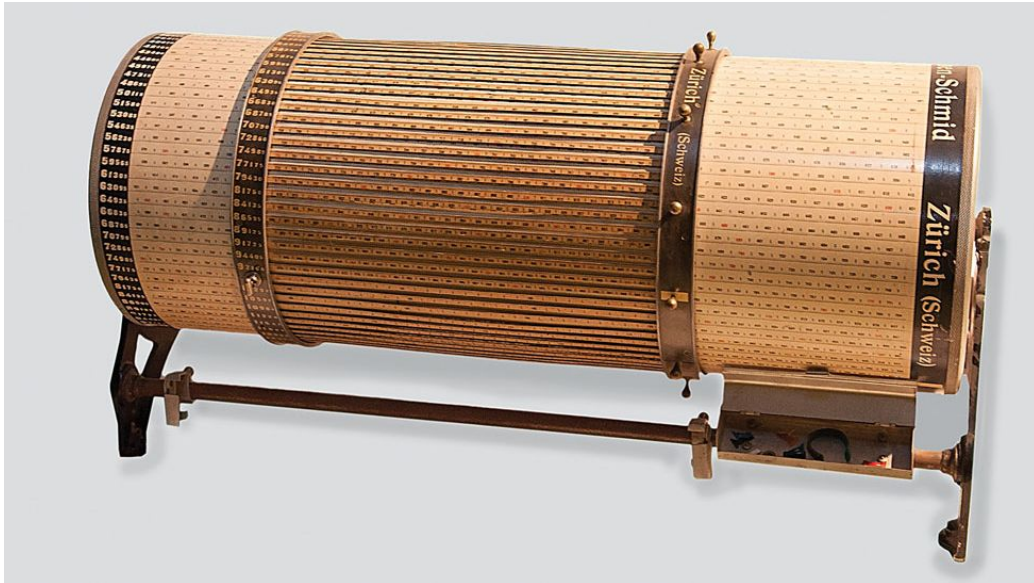
Figure 14: A 24 m LOGA cylindrical slide rule at UBS Basel. (picture provided by Céline Rader, UBS, reproduced with permission)
