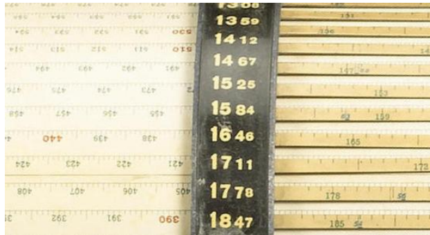
Figure 15: Detail of a 15 m LOGA cylindrical slide rule, with the grid wrongly mounted. ( http://www.bonhams.com/auctions/13633/lot/249 )
