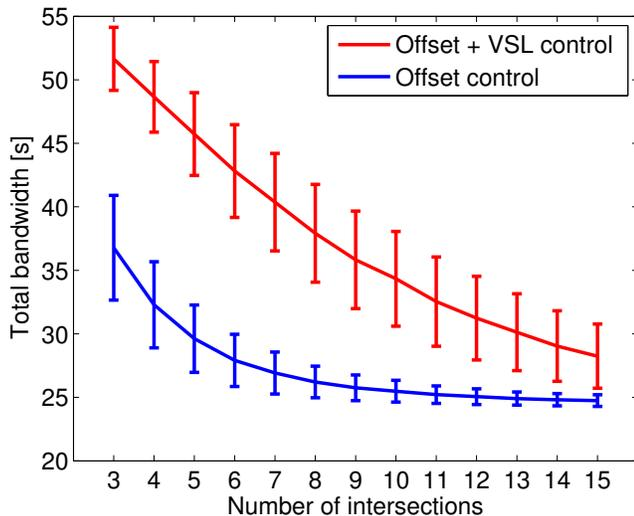
Fig. 2: Bandwidth degradation with number of intersections.
